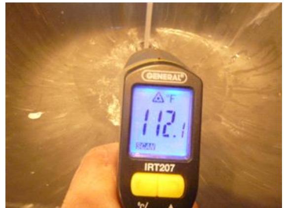
Hot Water Temperature 2nd Floor Bathroom Sink
